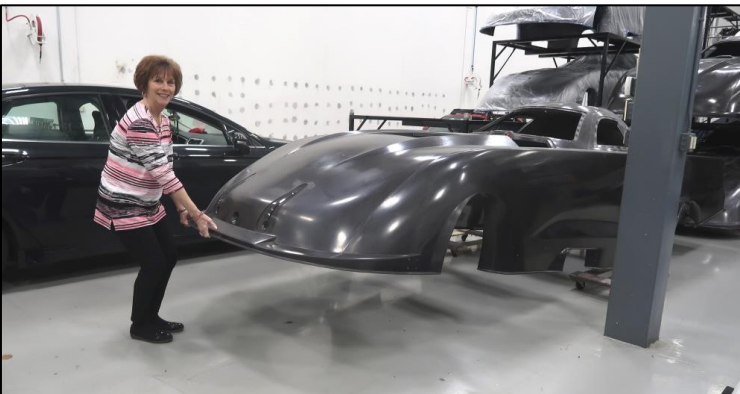
Club member Sue Lile picks up the carbon fiber body shell we get from Metalcrafters out of California. Sue doesn’t know it but those body shells cost $53,000 each (just the body shell alone ) and another $45,000 to turn it into a complete, race ready body. The shells weighs about 110 pounds and race ready weighs about 260 pounds. Each of the 2 funnv car teams has 2 complete bodv’s in the trailers.
